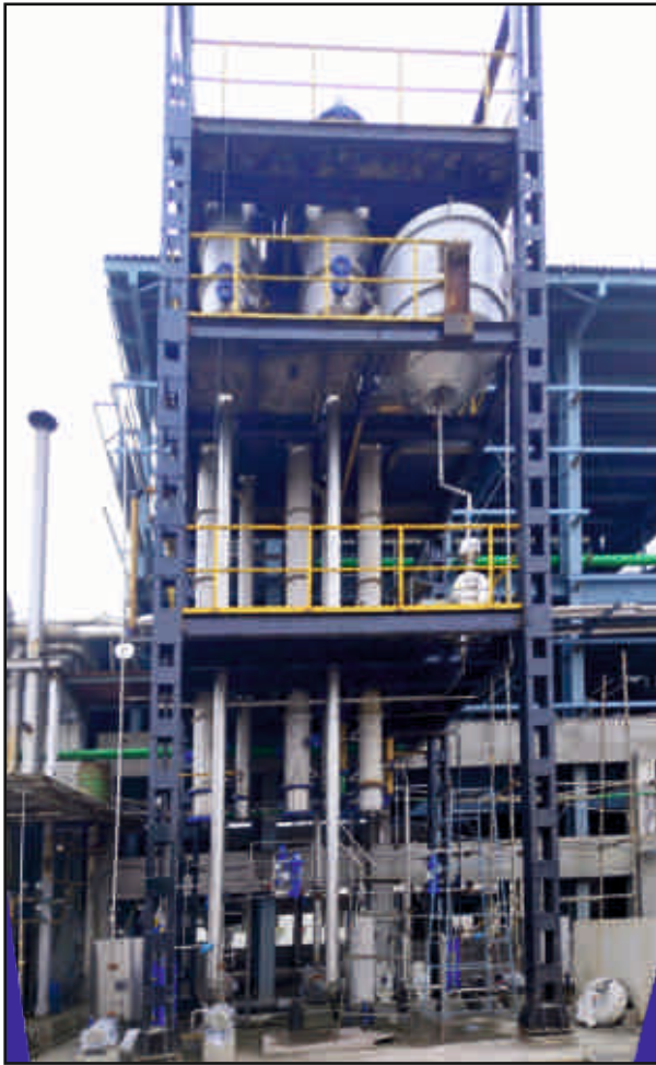
TWO EFFECT EVAPORATOR FOLLOWED BY PUSHER CENTRIFUGE FOR SALT SEPARATION
