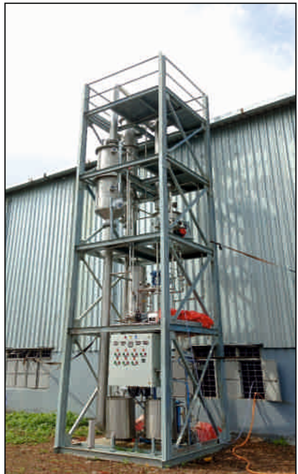
SKID MOUNTED SINGLE EFFECT EVAPORATOR FOLLOWED BY BASKET CENTRIFUGE FOR SALT SEPARATION
